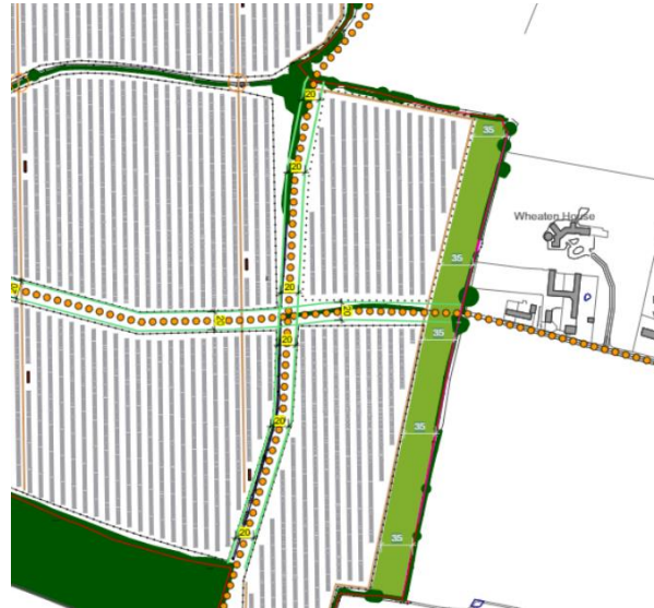
Proposed Site Layout Plan showing green buffer off-set from properties to the east
